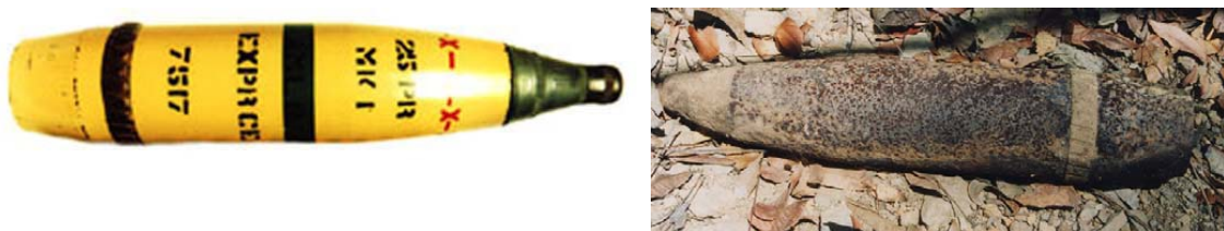
25 pdr HE fuze PD No 119 (left) and UXO fuze PD No 117 (right).
