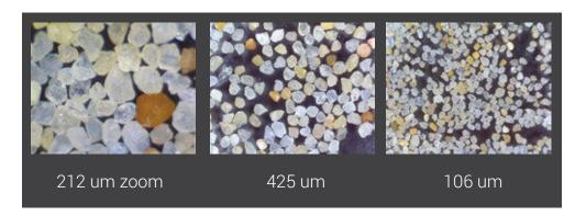
This excellent guartz sand is consistent and has good structural integrity. It will maintain structure throughout handling. There is no free clay or silt component under testing. The sand is rounded to sub rounded, essentially fine mainly siliceous, with guite hard, strong and durable fragments.
